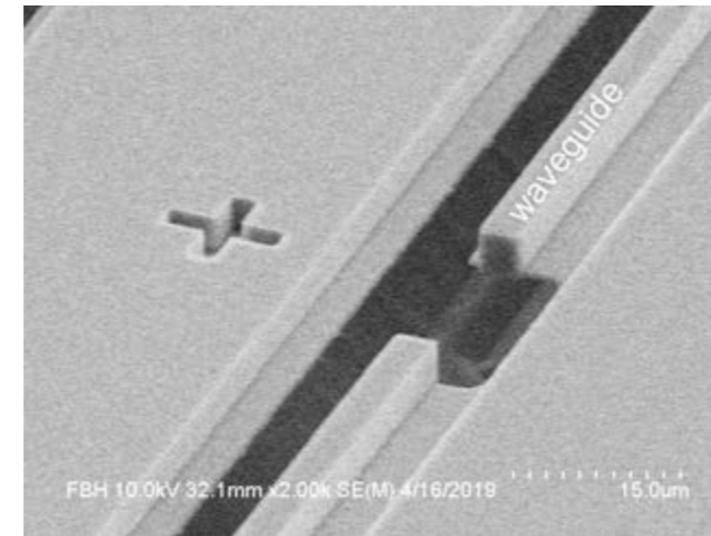
Fig. 2a. Inclined SEM view of a 4 \times 4 \mu\text{m}^2 intermittent waveguide with a gap of 12 \mu\text{m} . The waveguides were manufactured with an optimized process, allowing the use of dielectric materials of up to 4 \mu\text{m} thickness.
