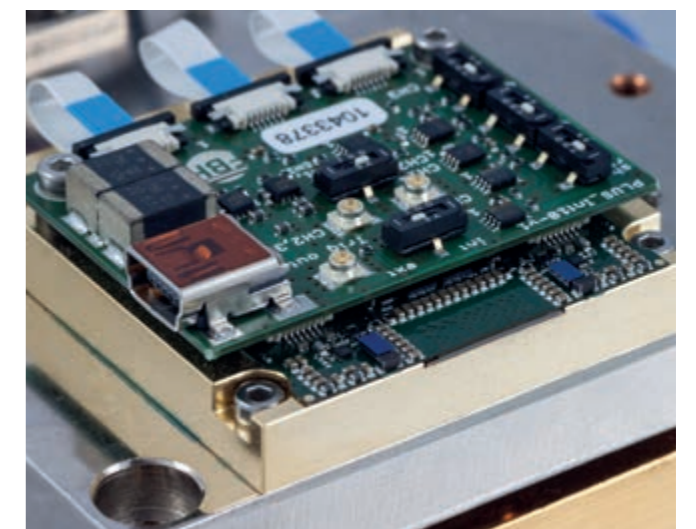
Fig. 4. Complete setup of the pulse laser module with laser diode, driver and interface circuit.
