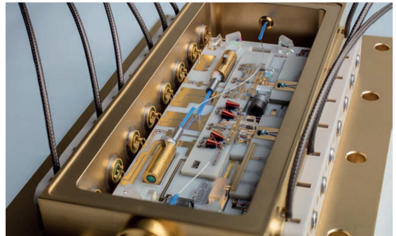
Fig. 3. Hybrid micro-integrated laser module (see p. 74), comprising a master oscillator power amplifier where a narrow-linewidth extended cavity diode laser acts as master oscillator. The emission is then amplified by a ridge-waveguide semiconductor chip.
