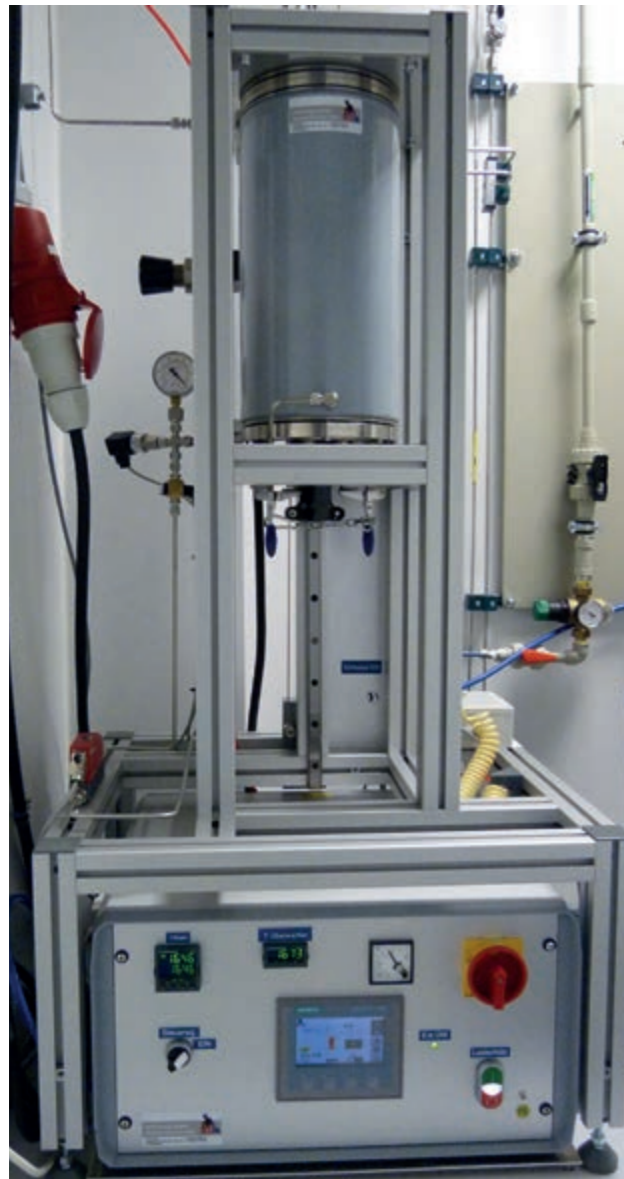
Fig. 1. Furnace for high-temperature annealing at FBH.
