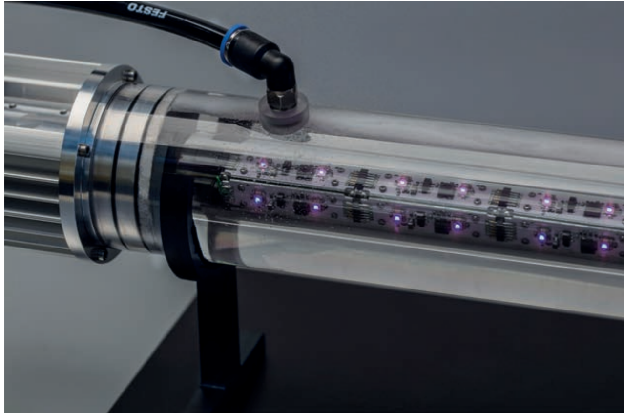
Fig. 1. Water disinfection module equipped with UV LEDs. Operation of the LEDs in the immediate vicinity of water recommends their protection by a hermetic package.
