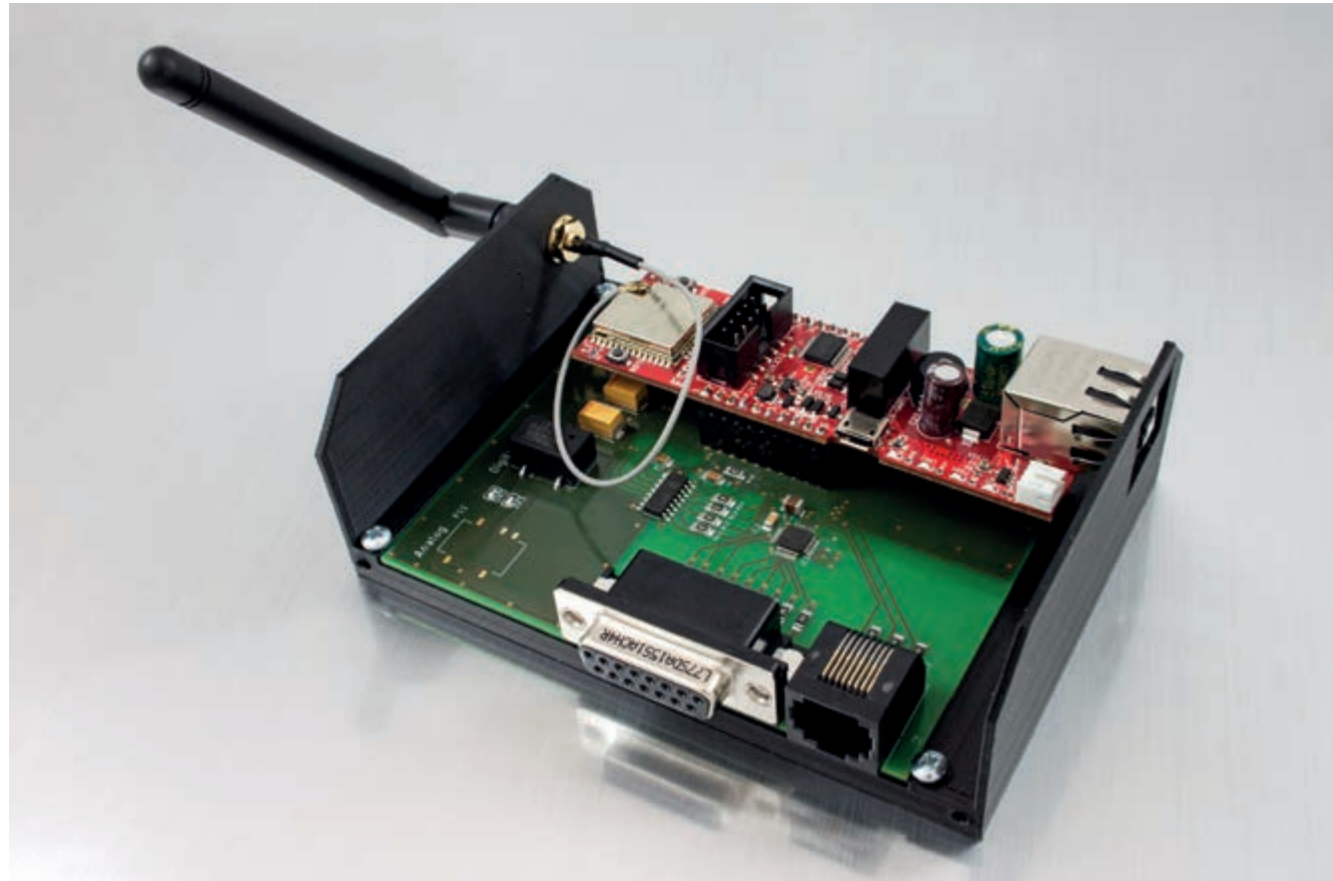
Fig. 1. Prototype of the iSensU IoT device with connectors for industrial light-tower read-out and additional 8 sensor inputs. Connectivity is achieved through WiFi, LAN (with PoE) or BLE.
